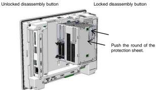
Procedure 3. Fix the expansion modules by pushing down the disassembly buttons to the same position as the expansion module's upper side.
