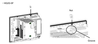
Procedure 5. Insert the A side of the mounting clamp into the groove. And hook the B side of the mounting clamp on the hole of the expansion module.
