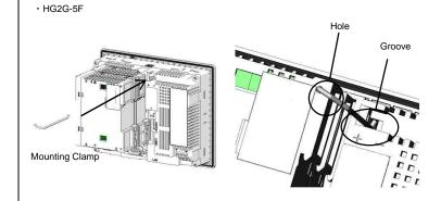
Procedure 6. Fasten the mounting clamp with the screw to a specified torque of 0.6  $\ensuremath{\text{N}} \cdot \ensuremath{\text{m}}$ pushing the mounting clamp as shown in the following figure. After fastening the mounting clamp, make sure that the mounting clamp is not loose and not having a gap.
