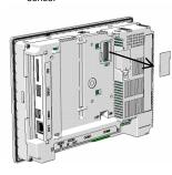
Procedure 2. Unlock disassembly buttons of expansion modules and then push the expansion modules into the back of the HG making sure of the position of the expansion
