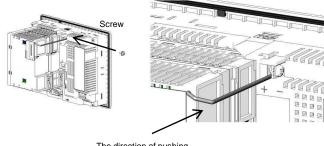
The direction of pushing the clamp
